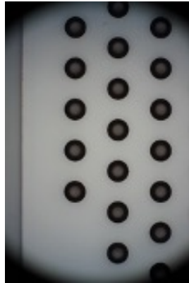
Figure 2a: Example of holes designed for optical fiber in a borosilicate glass after 100 cycles of temperature testing
